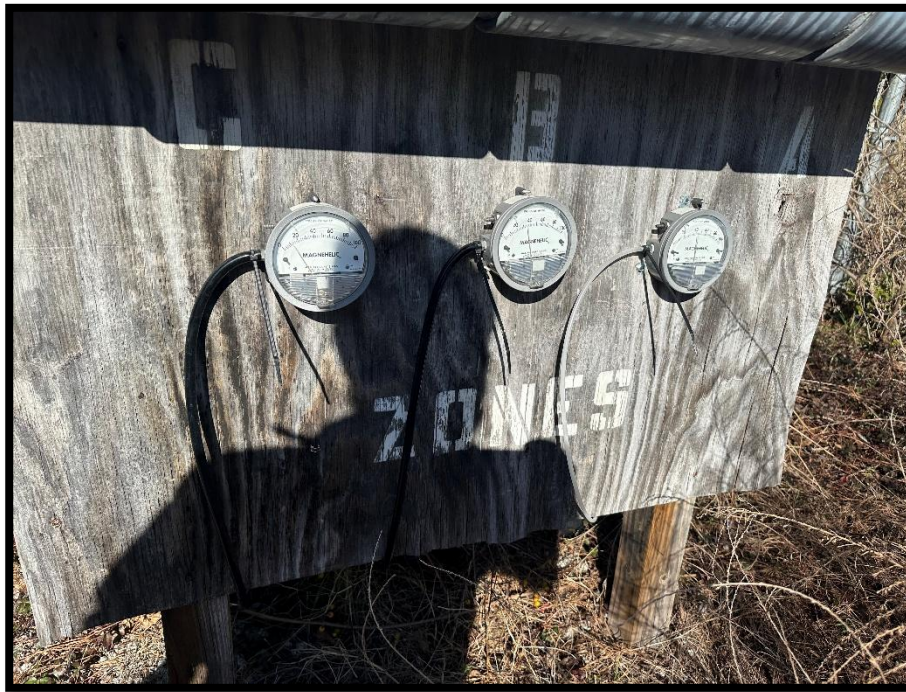
Photograph 25 – Vacuum Zones after Tube Replacement
