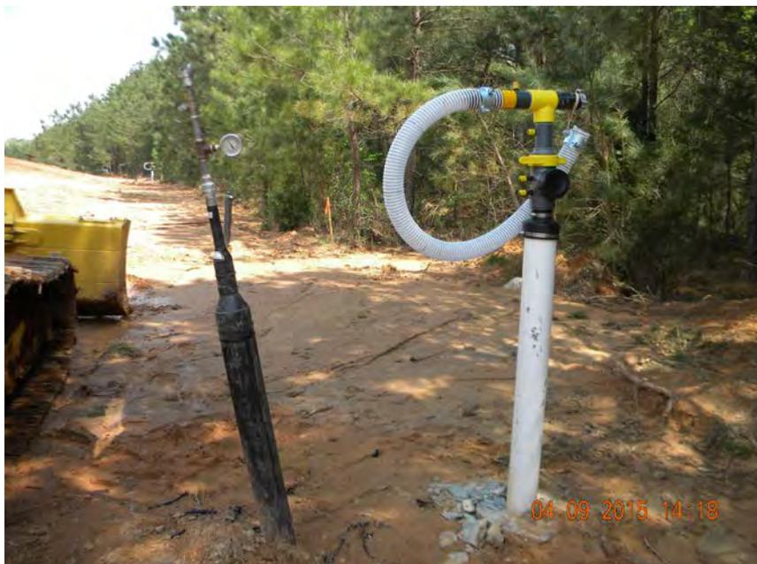
**Photo 10. Pressure gauge for pressure test of header pipe.
