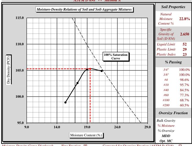
Moisture-Density Curve Displayed: Corrected for Oversize Fraction (ASTM D 4718) Fine Fraction 🗵 Sieve Size used to separate the Oversize Fraction: #4 Sieve 区 3/8 inch Sieve □ 3/4 inch Sieve □ Mechanical Rammer Manual Rammer X Moist Preparation □ Dry Preparation X References / Comments / Deviations:
