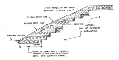
Benching and Keyway for Fill Slopes constructed along Existing Slopes
